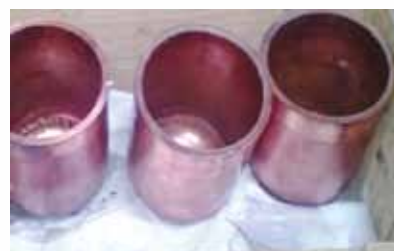
Combustion Chamber Inner Shell
