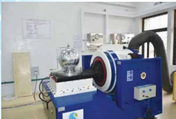
SPS-CAT: 4 Tonne Vibration shaker facility
