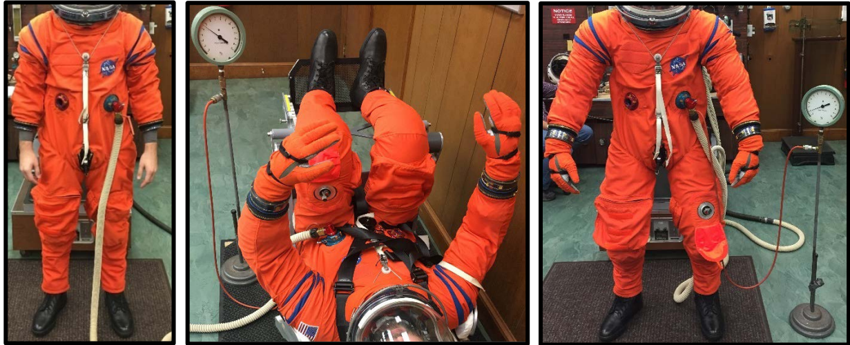
Figure 1. S1041 OCSS Suit Prototype. Unpressurized, at 4.3 PSID, and at 1 psid vent pressure
