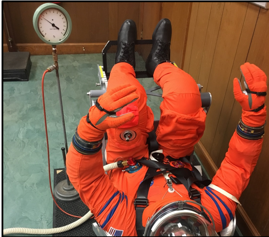
Figure 10. Manned pressurized (4.3 psid) testing of the OCSS suits, prior to VPIST2
