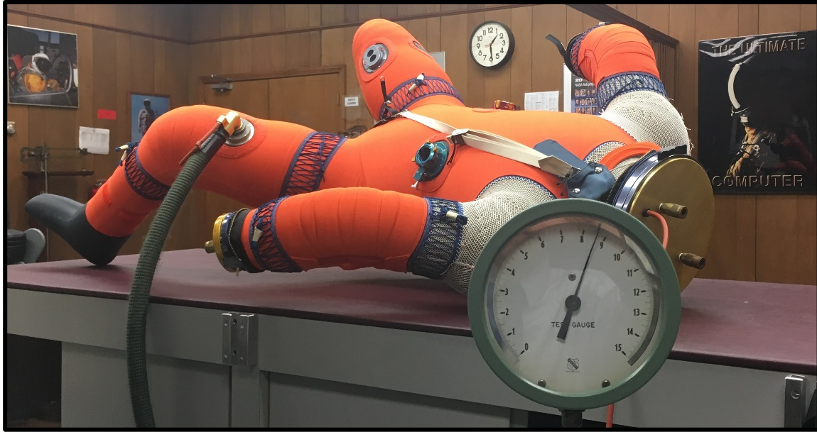
Figure 5. Structural testing at 8.6 psid
