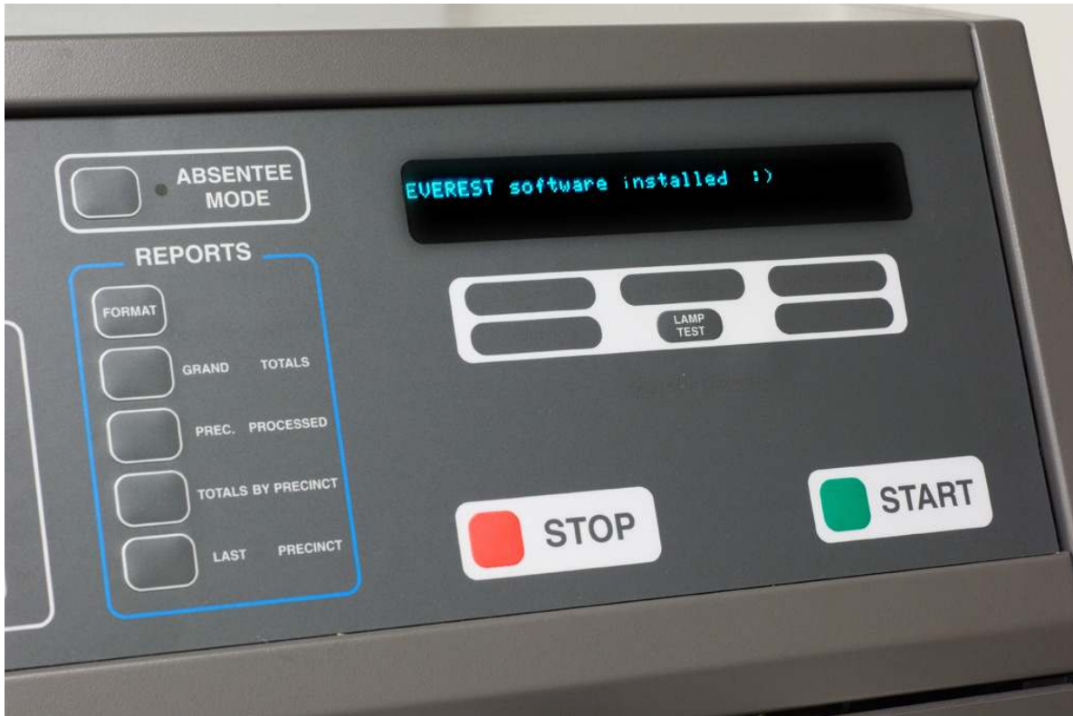
Figure 7.4: M650, with display controlled by forged firmware update disk
