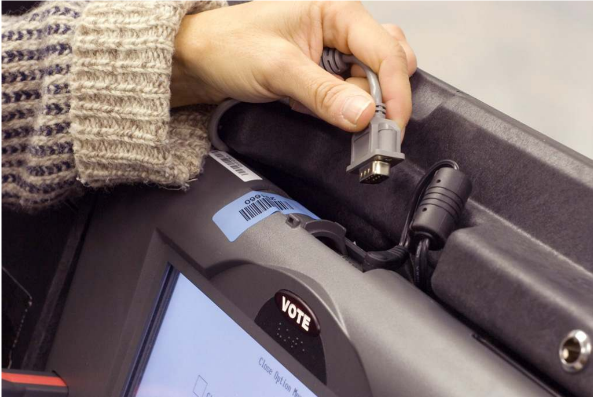
Figure 7.2: The connection to the RTAL/VVPAT printer port is physically unprotected
