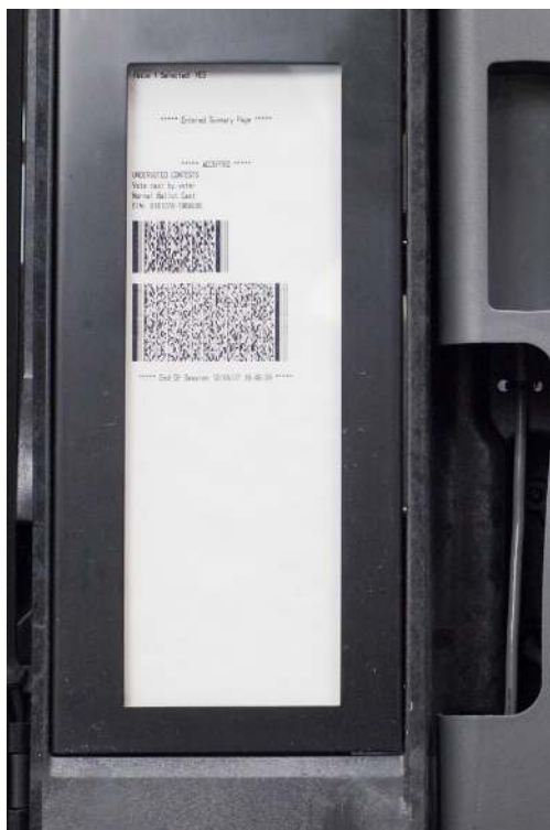
Figure 7.3: A VVPAT barcode encoding voter selections
