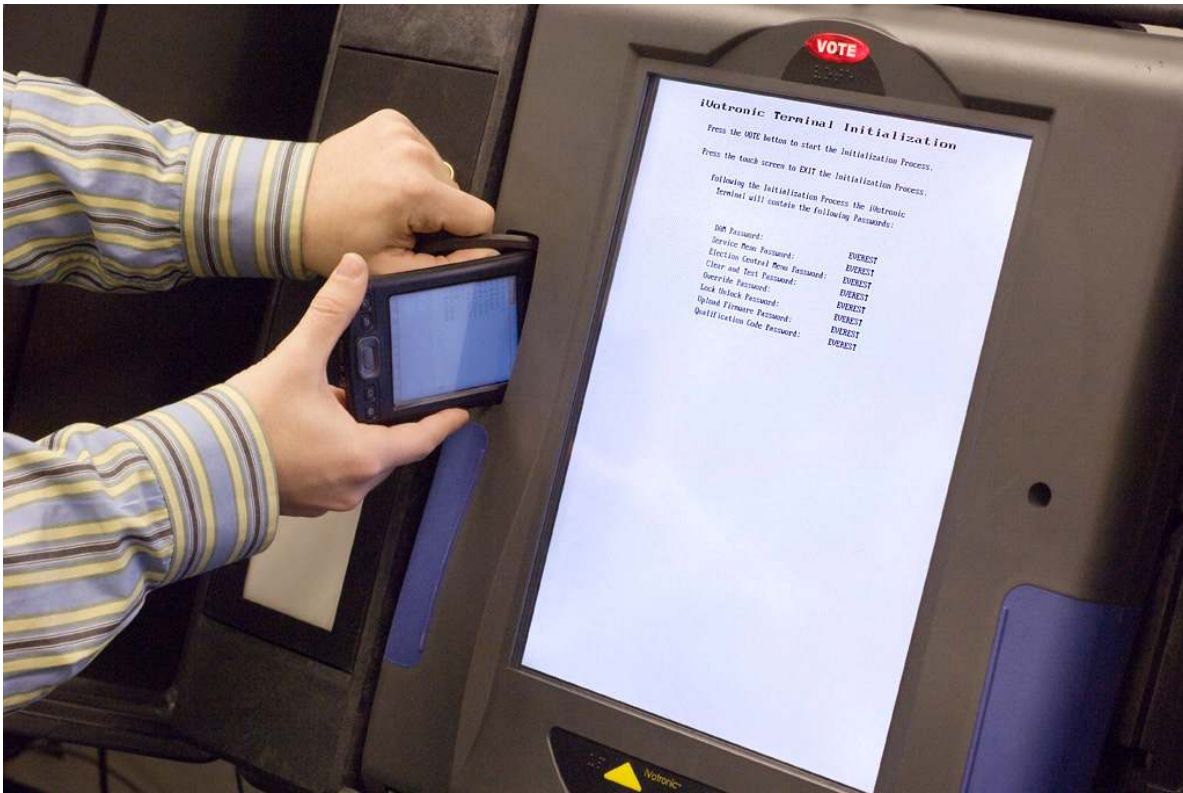
Figure 7.1: A PEB emulator running on a Palm Pilot simulates an initialization PEB during an open election, resetting all terminal passwords to “EVEREST”
