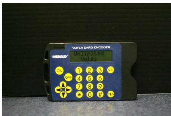
Figure 14.2: A Voter Card Encoder running arbitrary software.
