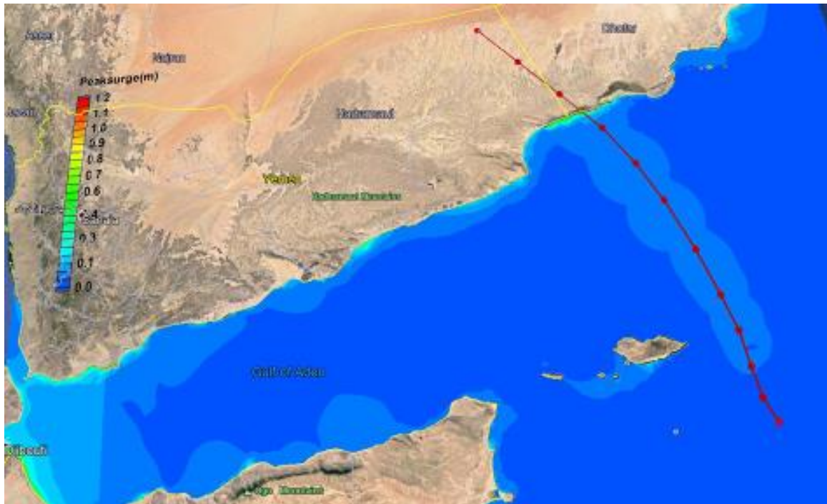
Fig. 3.3.7: Storm Surge Forecast issued by INCOIS ADCIRC Model based on 0600 UTC of 23 rd May, 2018
