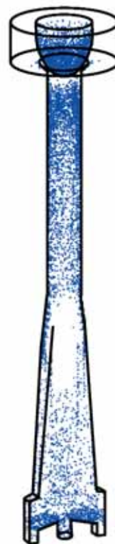
Figure 16 Final entrapment location of inclusions on stopper rod and nozzle walls (flow conditions in Figure 3).
