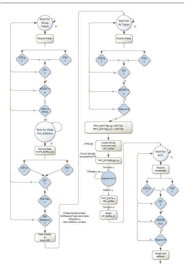
Figure 14 - Set Address state machine
