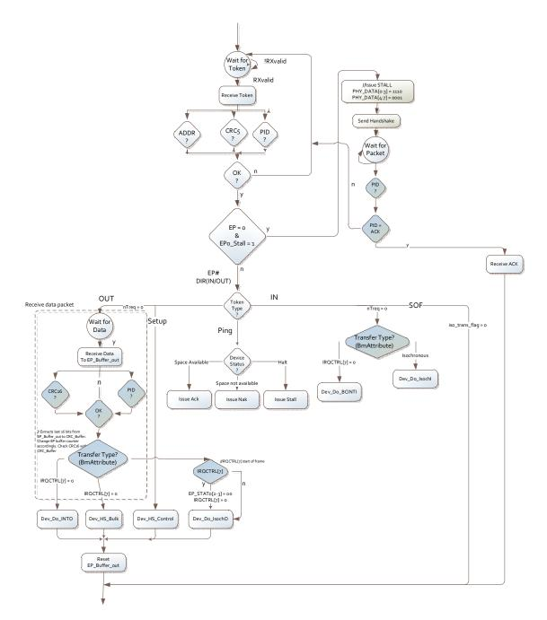
Figure 6 - Configured Final State Machine
