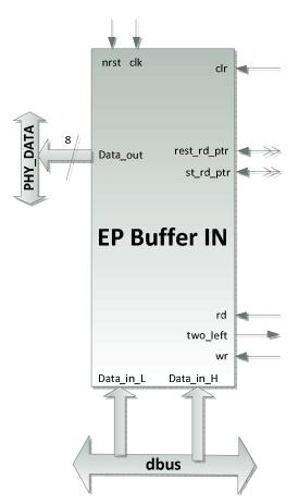
Figure 22 - EP Buffer IN module block diagram
