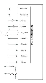
Figure 9 - UTMI Interface Block diagram.
