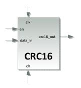
Figure 24 - CRC16 module block diagram
