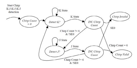
Figure 13 - High speed detection state machine
