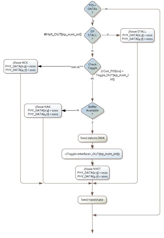
Figure 40 - Bulk OUT Transfer state machine
