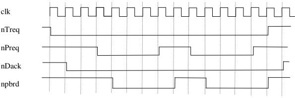
Figure 29– DMAC handshake signaling during an OUT transaction. Two packet transfers in one transaction.
