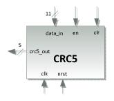
Figure 23 - CRC5 module block diagram
