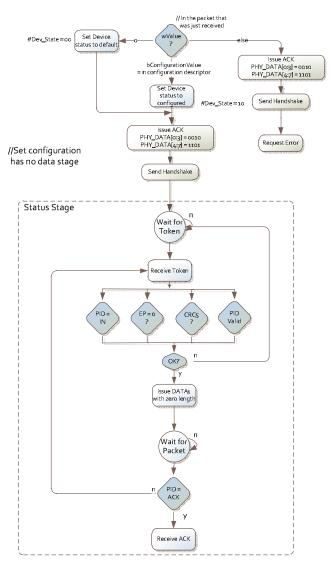
Figure 15 - Set Configuration state machine
