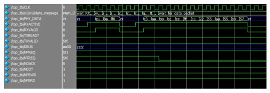
Figure 33 - Packet received from the UTMI in an OUT transaction.
