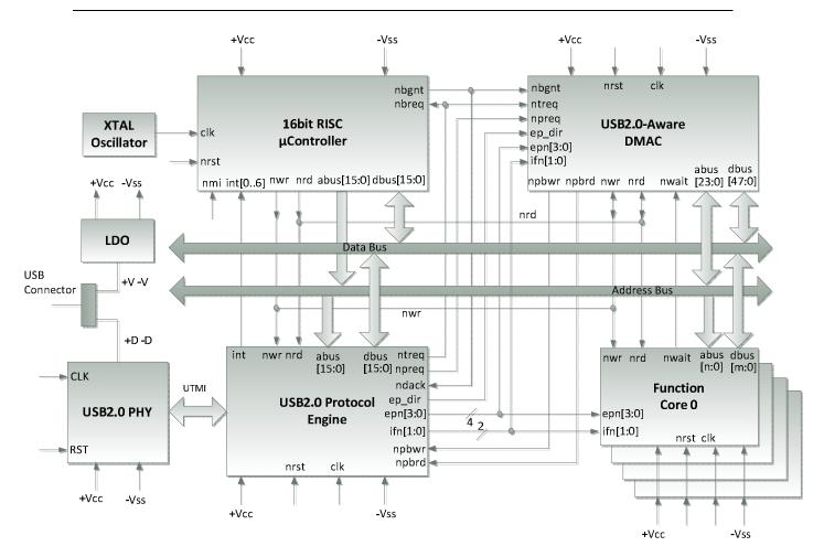
Figure 8 - µController-based Device Controller Block Diagram
