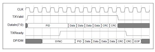
Figure 32 - UTMI transmit signals timing
