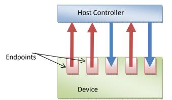
Figure 1– Each endpoint supports data flow in one direction: either input (from device to host) or output (from host to device).
