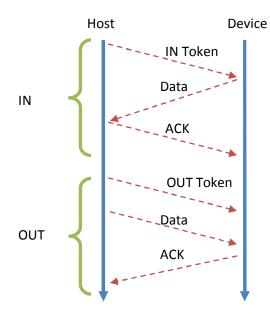
Figure 4 - A typical USB transaction involves a token packet followed by a data packet and ends with a handshake packet
