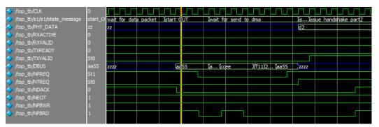
Figure 34 - Packet is sent to the DMA in an OUT transaction.
