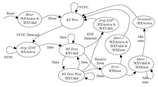
Figure 26- UTMI Receive State Diagram
