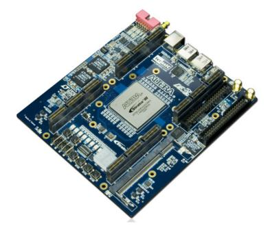
Figure 7 - Altera DE3 FPGA development board
