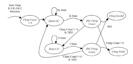
Figure 2 - High speed detection state machine
