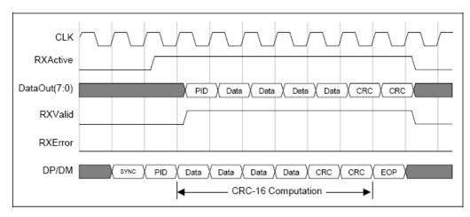
Figure 27- UTMI receive signals timing
