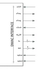
Figure 10 - DMA Interface Block diagram.
