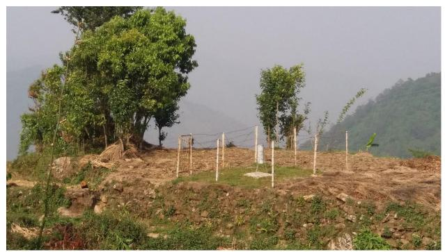
Figure: Rain Gauge Station
