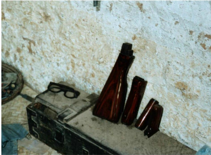
PLATE 7:33, The Weapons Workshops - The Process - Making the Wooden Stock - Painting and Varnishing 3
