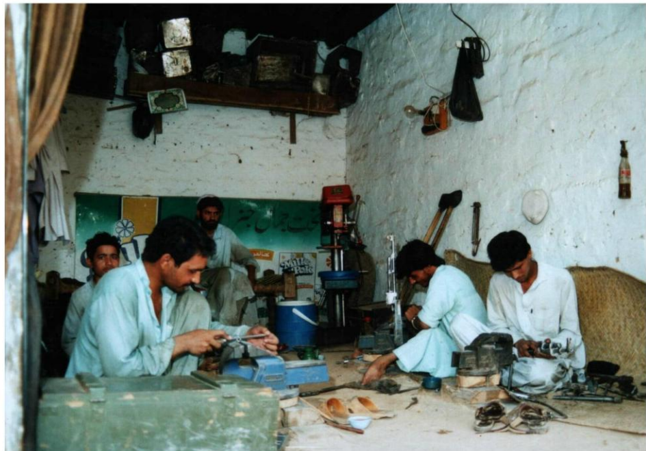
PLATE 7:48, The Weapons Workshops - The Process - Making the Breach Housing 7
