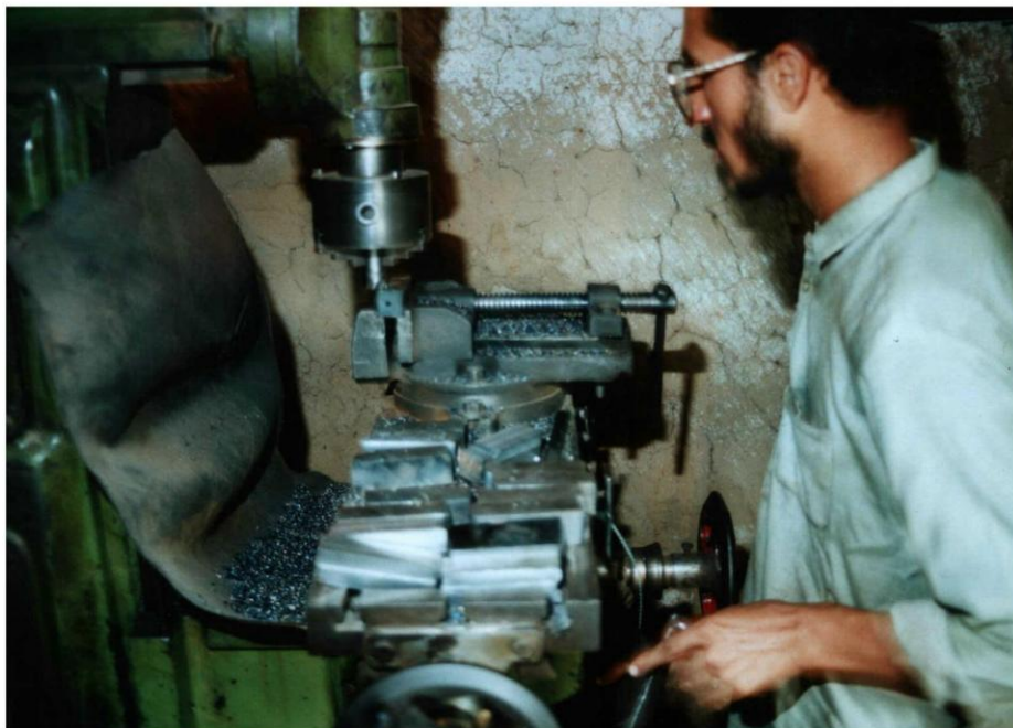
PLATE 7:42, The Weapons Workshops - The Process - Making the Breach Housing 1
