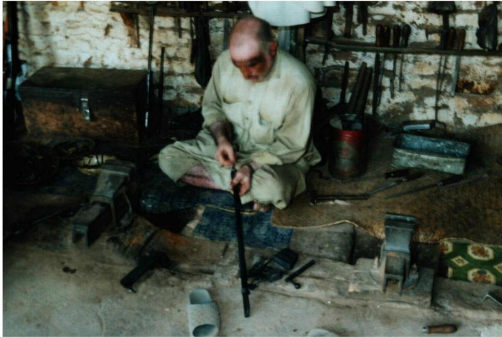
PLATE 7:41, The Weapons Workshops - The Process - Making the Barrel - Boring
