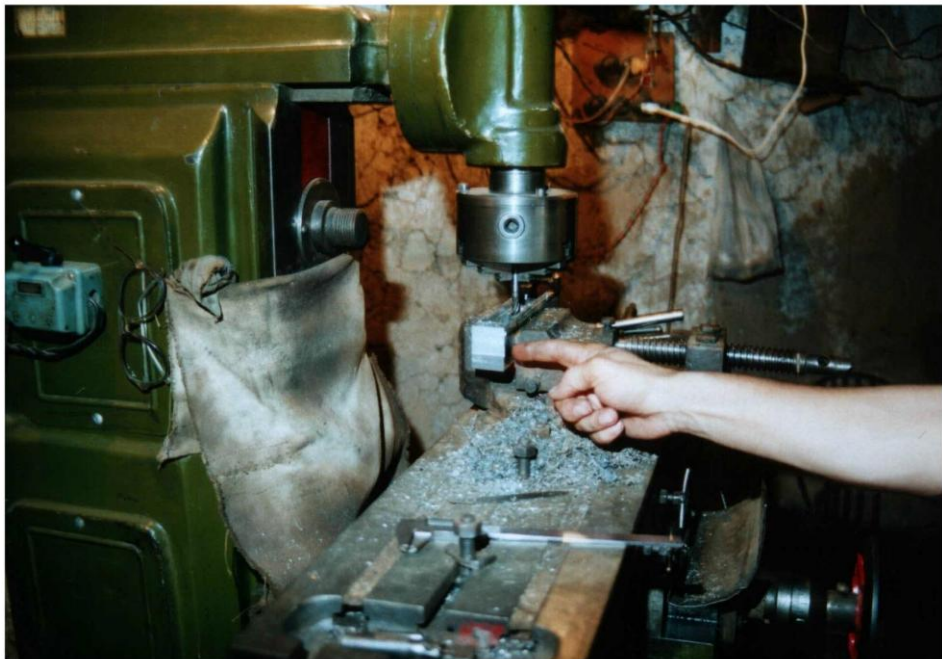
PLATE 7:44, The Weapons Workshops - The Process - Making the Breach Housing 3
