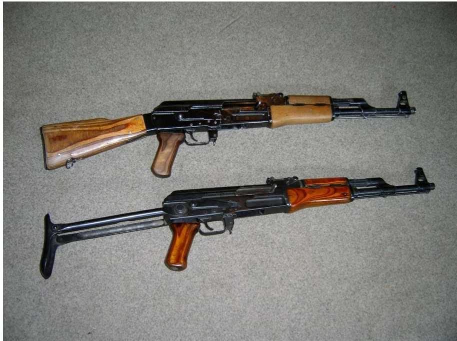
PLATE 7:54, A comparison between the much recognised AK-47 (top) and the folding stock Kalacov (bottom) derivative made in 'Darra'. There is relatively little outward difference between the weapons.
