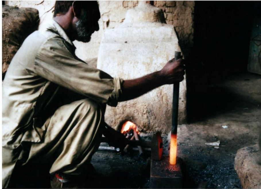
PLATE 7:35, The Weapons Workshops - The Process - Making the Barrel
