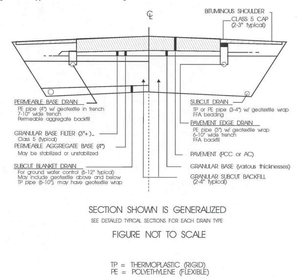
Figure 5-4.1. Typical sections, subsurface drainage.
