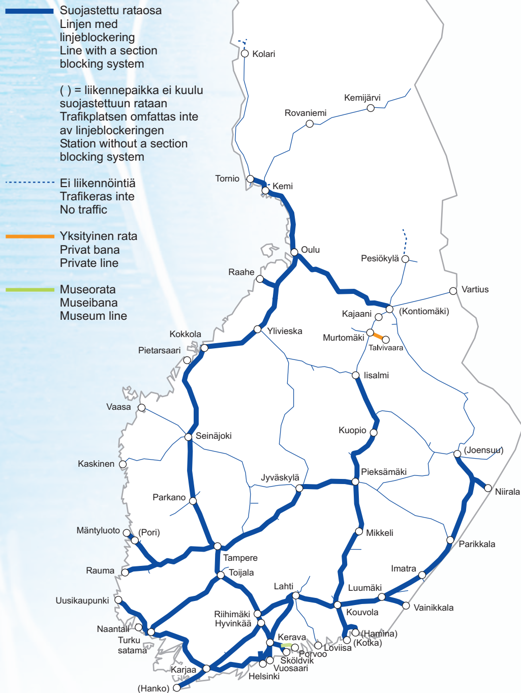
Figure 1. Lines with a section blocking system.
