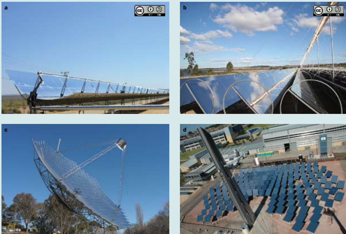
Figure 10.24 The four types of solar thermal concentrators: (a) parabolic trough, (b) compact linear Fresnel reflector, (c) paraboloidal dish, and (d) power tower
