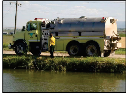
Figure 4. To minimize risk of engine water leakage through foot valve, prime with water from the drafting source rather than from the tank.
