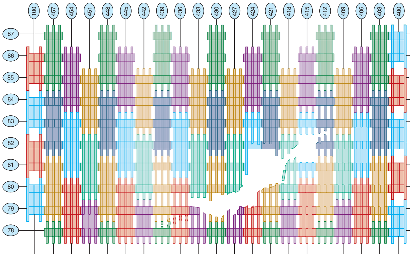
Figure 2-26 Impact damage to the south and east faces of WTC 2.
