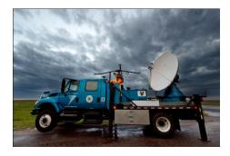
Tornadoes occur infrequently and often form very near the ground, making them difficult to measure with traditional stationary meteorological radars. Doppler On Wheels (DOWs) are mobile Doppler weather radars mounted on trucks that bring radars directly into the path of storms, allowing researchers to study them with greater accuracy and detail. These vehicles have allowed scientists to create the first ever
