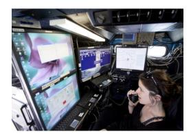
In addition to a large, rotating radar dish and an impressive antenna, the DOW vehicles have a radar operations "cockpit" that visitors can climb into. Depending on availability, the DOW team may also bring additional mobile weather measurement tools (tornado pods, weather balloons, disdrometers (used to measure precipitation, etc.).
