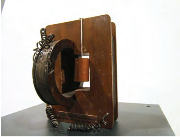
Rotating field realization (courtesy of Museum of Electrical Technology, University of Pavia)
