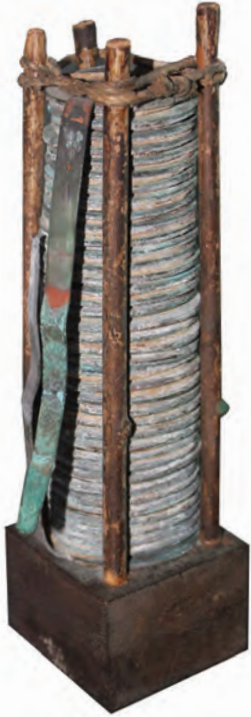
A replica of Volta's pile. The original was destroyed in the fire of the 1899 Universal Exhibition; what shown here is a copy made in 1899.
