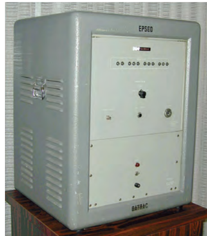
1954 “DATRAC” 11-bit, 50-kSPS Vacuum Tube ADC Designed by Bernard M. Gordon at EPSCO. (With the permission of Analogic Corporation, Peabody, MA.)
