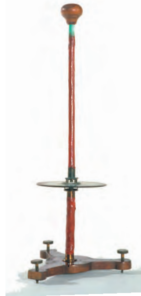
The original early 19th century disc condenser kept in the Museo della Storia, University of Pavia.
