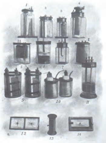
Four series of the first century of piles/batteries. On the top-left (1, 2, 3, 4, 5, 6, 7, 9, 10, 11) various versions of the Leclanché pile – From 1899 Como e l'esposizione Voltiana , N. 7, July 1, 1899
