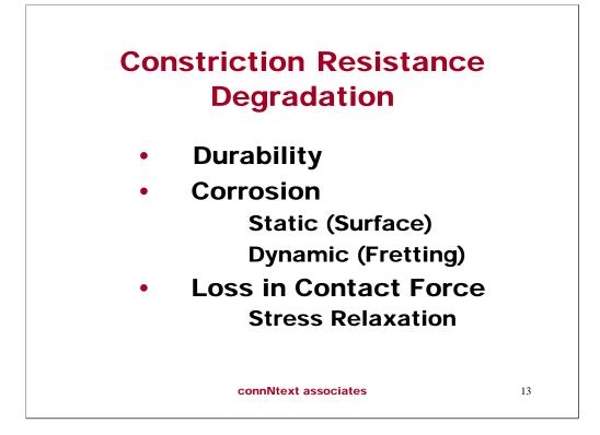
Durability refers to the wear that takes place during mating of the connector and can result in the loss of the contact finish and the finish properties that were designed in to enhance the connector performance. Durability depends on the finish material, the contact geometry and the contact force - materials/design parameters - and the number of mating cycles the connector must support - an application parameter.
