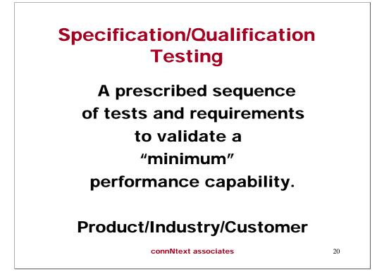
S/QT requires better definition of protocols. The test sequence and requirements may be defined by the connector manufacturer in a Product Specification or in a Standards document by a industry group such as EIA, TIA, IPC etc. in the US or by the ISO or IEC in international standards. A Corporation may also issue its own specification such as Bellcore/Telcordia 1217.
