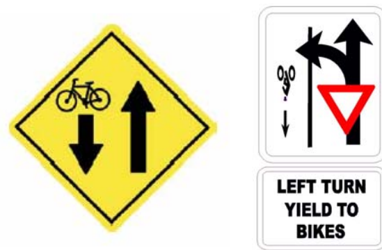
Figure 16: Example Contra-Flow Signage.
