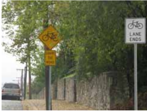
Bike Lane Ends Sign Used With Share the Road Sign in Nashville
