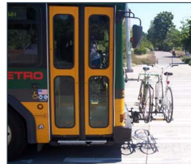
King County Metro bus bicycle racks currently have room for two bicycles.
