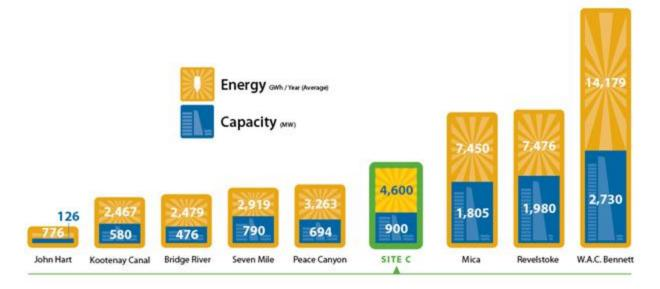
Figure 12: A comparison of the electricity generation capabilities of the proposed Site C hydroelectric facility with BC Hydro's largest hydroelectric facilities. Source: (BC Hydro, 2007).
