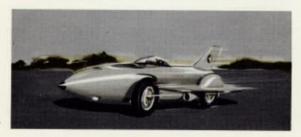
plastic reinforced with glass fiber made it possible to produce special forms without the terrific die expense of metal bodies. They were made strictly for experimental and exhibit purposes, but one—the Chevrolet Corvette sports car—so took the public fancy that it was put into limited production in 1953.
