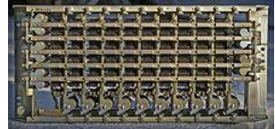
Type B (1960) Western Electric 100-point 6-wire crossbar switch
