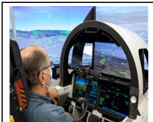
Shown here is the X-59's eXternal Vision System, which is a forward-facing multi-camera that enables the pilot to "see" what is in front of the vehicle's elongated nose.
