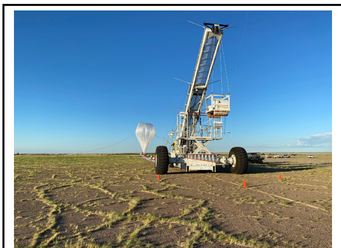
The JPL-SLS instrument is a passive submillimeter wave radiometer measuring gases in Earth's stratosphere such as ozone, ClO, BrO and HO 2 . This photo reflects the launch configuration with the Balloon Program Office Mobile Launch Vehicle "Big Bill." -Credit NASA 28 Aug 21.
