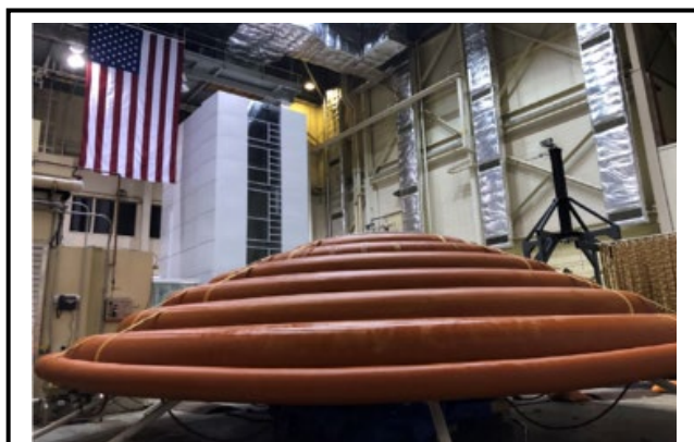
The Low-Earth Orbit Flight Test of an Inflatable Decelerator (LOFTID) is a partnership between NASA's Space Technology Mission Directorate and the United Launch Alliance (ULA) and is poised to revolutionize the way NASA and industry deliver payloads to a planet's surface or into orbit, utilizing aerodynamic forces instead of propulsion. LOFTID is scheduled to launch from Vandenberg Air Force Base in late 2022. This image shows LOFTID inflated in Building 1250 at LaRC.
