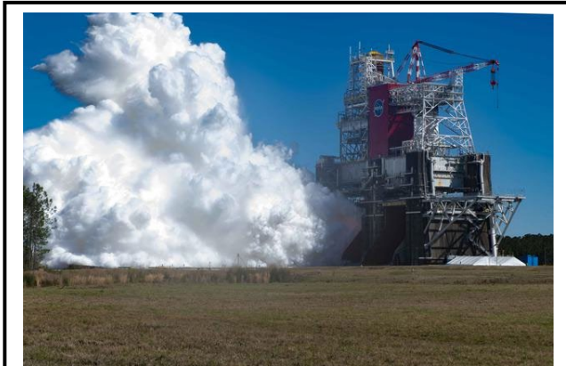
The core stage for the first flight of NASA's Space Launch System rocket is seen in the B-2 Test Stand during a second hot fire test, on Thursday, March 18, 2021. This took place at NASA's Stennis Space Center near Bay St. Louis, Mississippi. The four RS-25 engines fired for the full-duration of eight minutes during the test and generated 1.6 million pounds of thrust. The hot fire test is the final stage of the Green Run test series, a comprehensive assessment of the Space Launch System's core stage prior to launching the Artemis I. mission.
