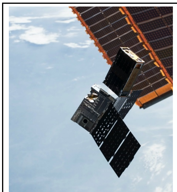
The TEMPEST-D CubeSat is pictured above shortly after being deployed into low-Earth orbit (LEO) from the International Space Station (ISS) on July 13, 2018. Slightly larger than the average shoebox, the TEMPEST-D mission lasted for nearly three years (de-orbited in June 2021) and paved the way for a future constellation of compact microwave sensors that could improve the temporal resolution of weather and climate data.
