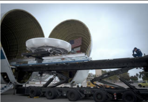
The Artemis IV Orion heat shield skin is offloaded from the Aero Spacelines Super Guppy to the K Loader at Moffett Federal Airfield on November 9, 2021
