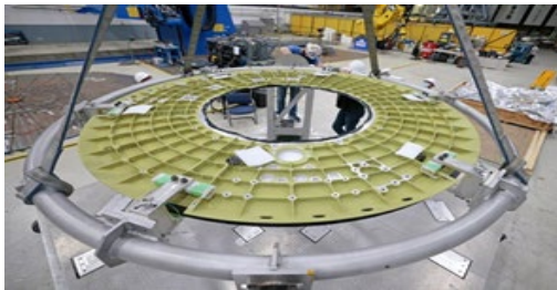
Top view of the Artemis IV CM pressure vessel forward bulkhead at Michoud Assembly Facility (MAF).
