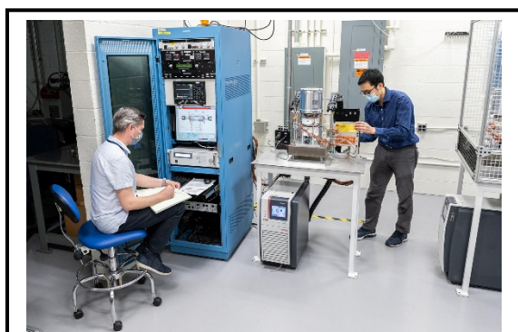
Shown above is the Sunpower Robust Stirling Converter testing at the NASA Glenn Research Center's Stirling Research Laboratory, a possible power conversion solution for the Dynamic Radioisotope Power System, which will enable future missions to use much less Pu-238 to produce the same amount of power.
