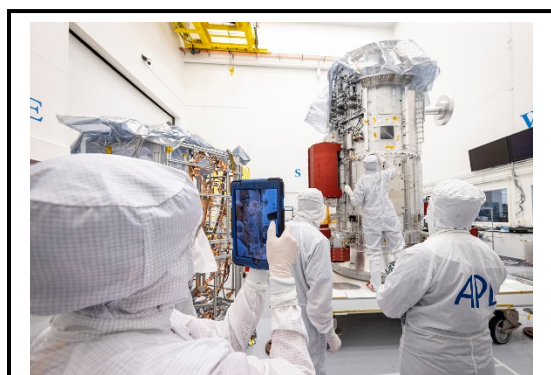
Flight hardware for the Europa Clipper mission is coming together at an increasing pace. Pictured above is the propulsion module containing the fuel tanks and engines. An additional module containing the electronics vault, the instruments, and the communications system will be placed atop this module, bringing the total height to more than 15 feet. With its solar arrays deployed, the spacecraft will span the length of a basketball court.
