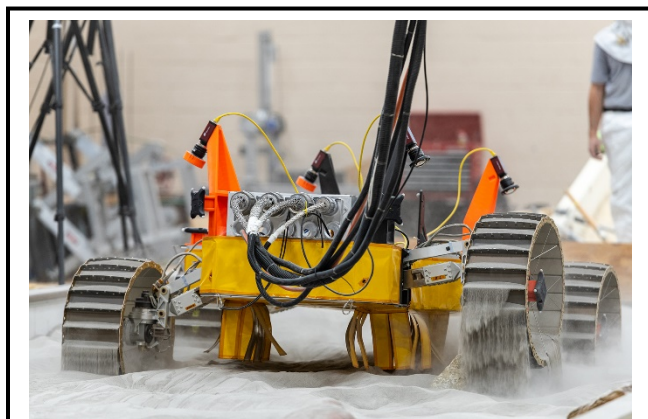
Shown here is the VIPER Rover in motion performing obstacle testing at NASA-GRC.
