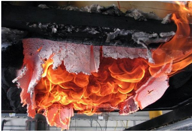
Figure 6: Specimen removal from furnace
