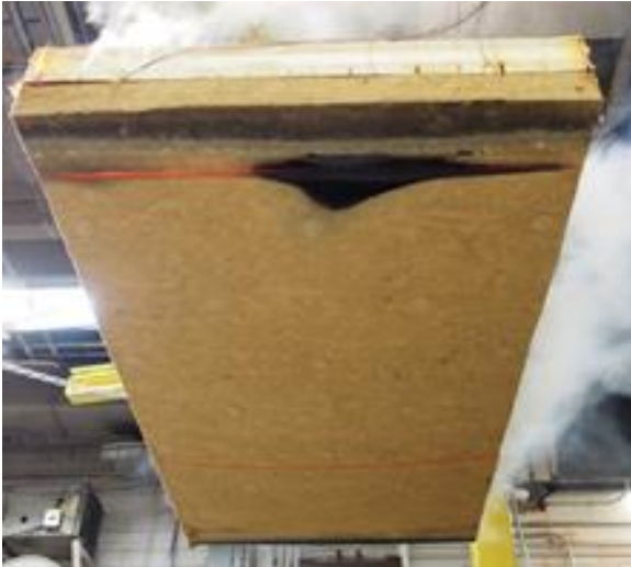
Figure 8: Specimen I-5 after removal from furnace
