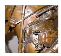
Another important type of decorative and protective surface often applied to copper alloy objects is patina. A patina is a thin, chemically-induced layer of relatively stable corrosion on the surface of an object. While patinas can form naturally over time, they are often intentionally created as a part of the finishing process. Patinas can be
