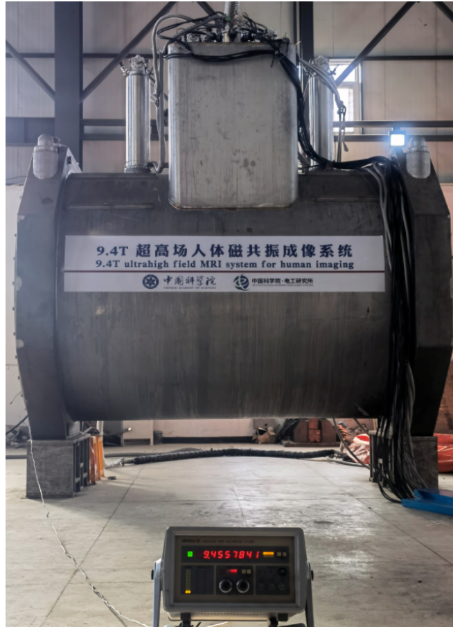
Fig. 3 Magnetic field value measured by a Metrolab PT2025 NMR magnetometer
