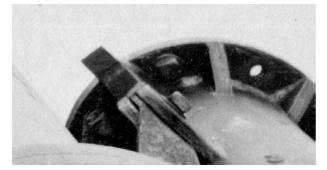
12 Conical taper on broken strut lug with intact upper lug joint in foreground
