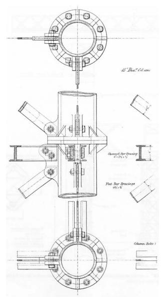
9 Line drawing of various joints on fifteen inch diameter column, including upper and lower lugs, strut, and flange, all cast as one with the column (Institution of Civil Engineers)
