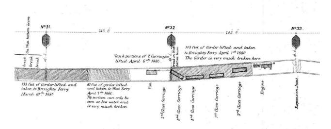
6 Plan of the section of the high girders between the fourth (no. 32) and fifth (no. 33) piers, showing the nearly intact train with the 4-4-0 locomotive at the front
