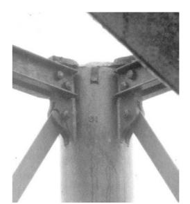
14 Closeup of fractured lug on third pier (looking west). Only one wing of the lefthand lug has broken, suggesting cyclic loading during or before the accident and collapse of the tower. There are no washers on the strut bolts, and these appear to be tightened by different amounts (judging by differing thread heights above the nuts)
