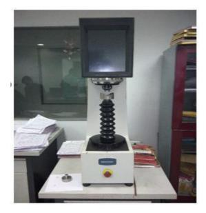
Fig. 3 Brinell hardness tester
