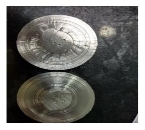
Fig. 4. Specimen after hardness test
