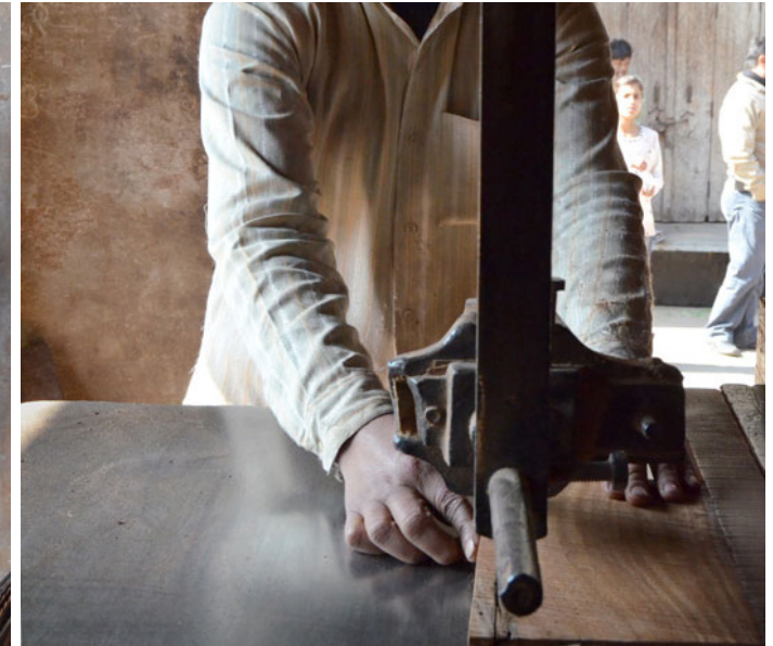
Slab being cut into smaller pieces.
