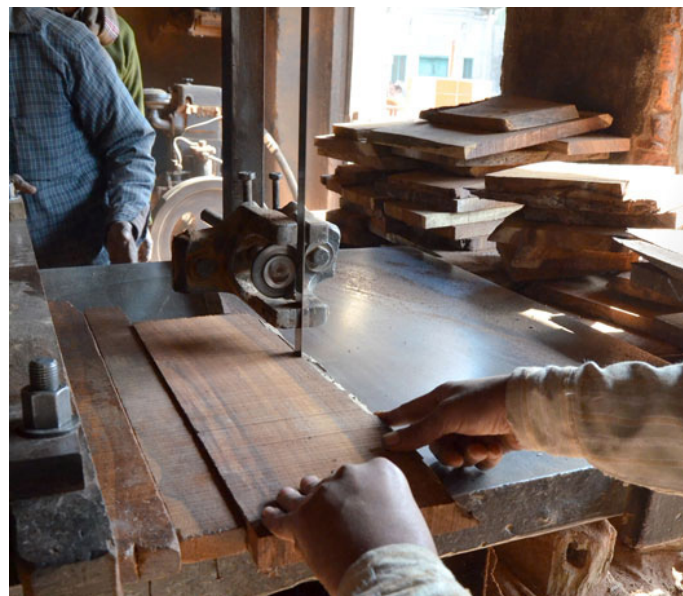
Slab being cut into smaller pieces.
