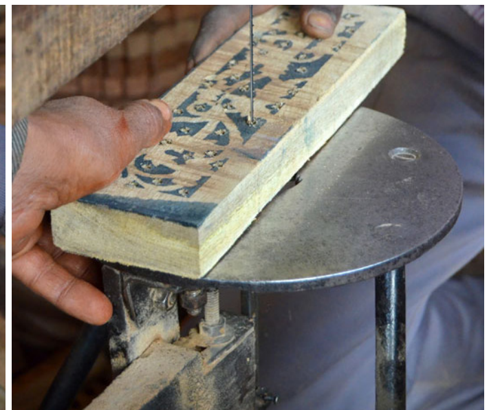
Holes being drilled for carving out the negative spaces.
