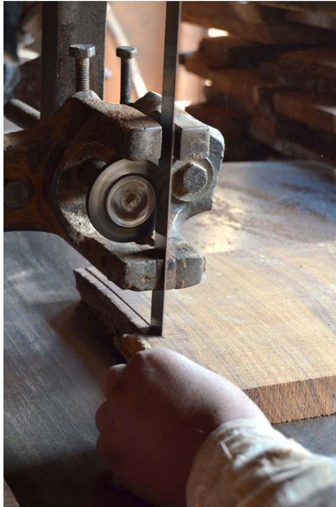
Slab being cut into smaller pieces.
