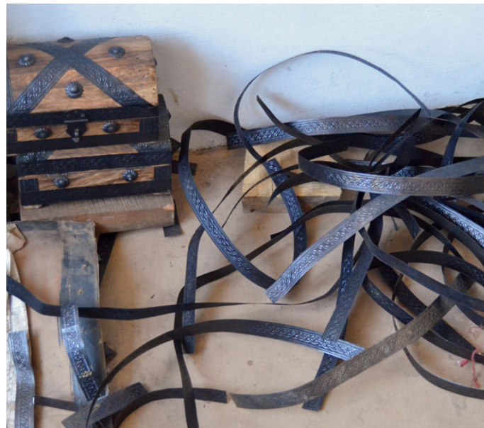
Black painted metal strips to be nailed on the boxes.
