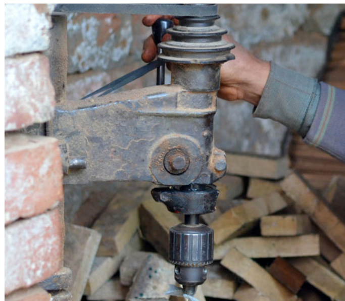
Holes being drilled for carving out the negative spaces.
