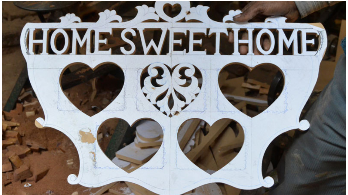
Design drawn on paper and stuck on wood for carving.
