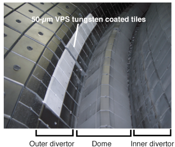
Fig. I.2.1-2 Tungsten coated tiles installed in the outer divertor.
