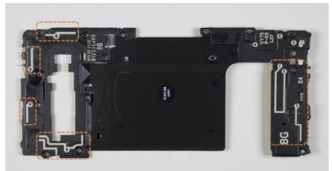
Figure 107: LDS antenna on Samsung
