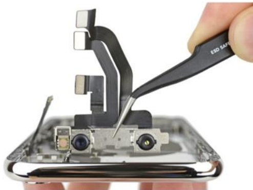
Figure 106: LCP antenna on iPhone
