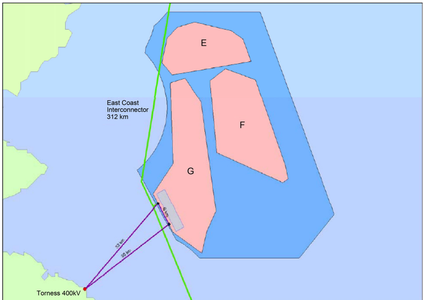
Fig. 4. Firth of Forth zone connection overview. The figure shows the two potential connection routes to the 400 kV substation at Torness. Polygon E represents Phase 1 of development and connection, followed by G (Phase 2) and then F (Phase 3).
