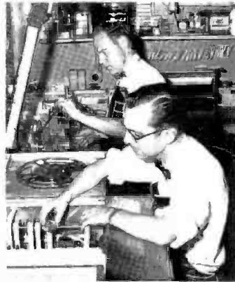
Film Laboratory — Fred E. Foshey, Jr., Staff Photographer, checks temperature of solution in Bridgamatic 16 mm film processing machine. This machine develops movie film at a rate of 100 ft. every five minutes. In background Frank Wildenhain prepares film just processed for show.
