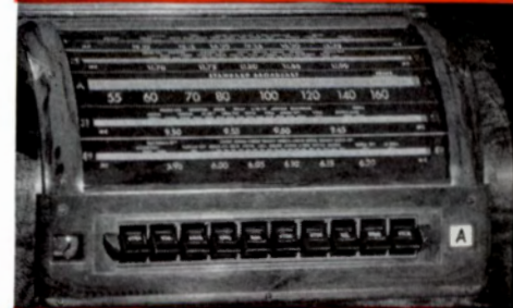
Electric tuning, Water-fall type of Overseas Dial offered in model 11Q4. Incorporates the new piano-key push buttons for electric tuning or switching to manual tuning, or an Electrola Attachment.
