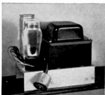
AC type of Power Supply Unit for Q Models
