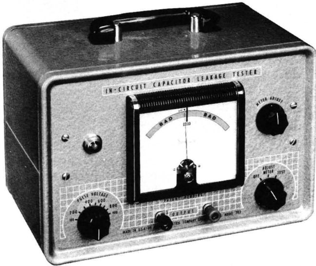
Fig. 6-6. Simpson in-circuit capacitor checker.
