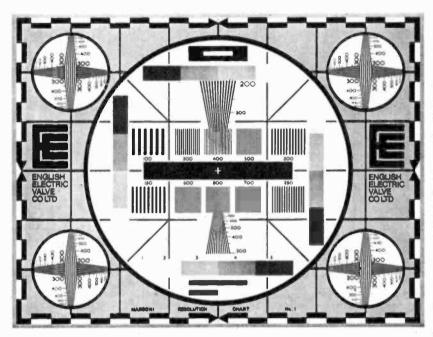
The English Electric Valve Company has recently produced a camera tube and system test chart specially for use with closed-circuit television (CCTV) systems.
