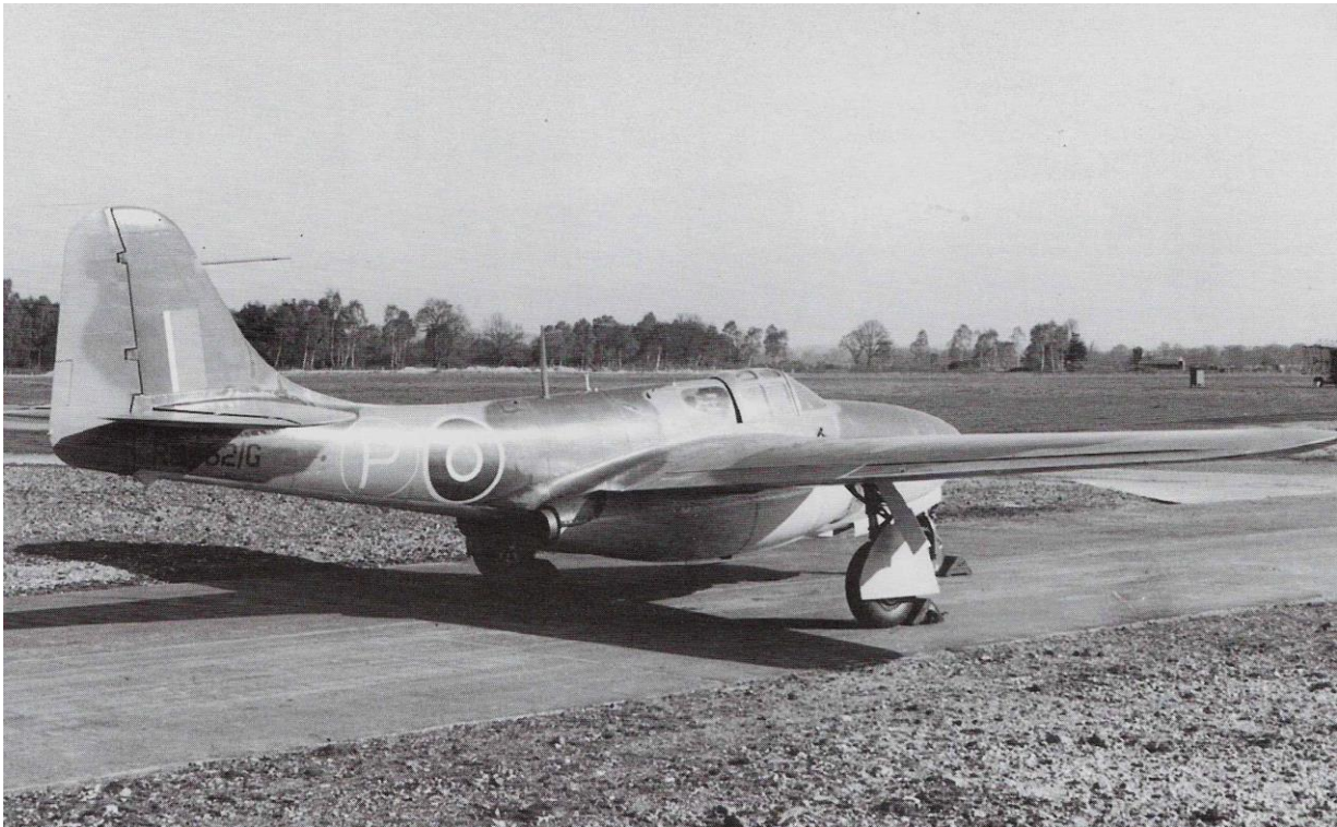
Figure 32 Bell XP-59A, two Whittle/GE engines
