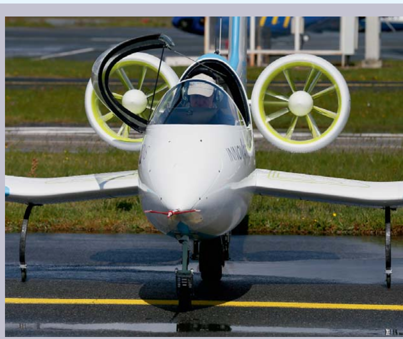
The E-Fan is a technology demonstrator of a fully electrically-powered, all-composite general aviation training aircraft.
