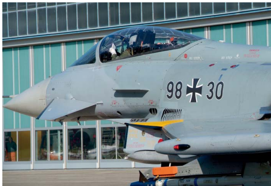
The new strakes and other AMK modifications will increase the Eurofighter's maximum wing lift, angle-of-attack limit and the roll rates at high angle-of-attack.
