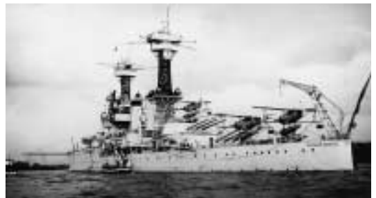
Curtiss scout aircraft aboard the battleship Tennessee. From the earliest times, people recognized that air superiority over a sea battle would yield an enormous advantage in spotting the fall of shot from observation aircraft flown from catapults on battleships. Jerome Hunsaker did vital work in developing practical catapults for this purpose.
