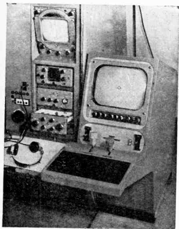
Fig. 3. Remote control console. The two large knobs control focus and zoom (left) and tilt and pan (right).
