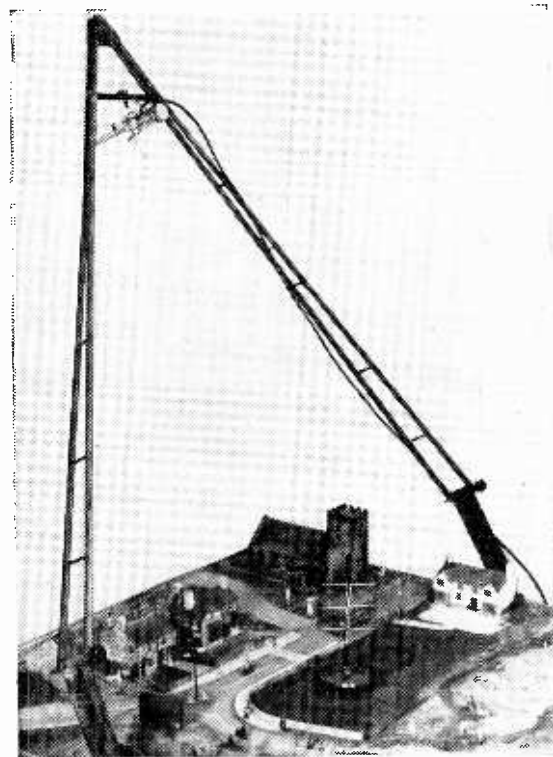
Fig. 3. The 3,000-Mc/s model aerial testing table (scale 4mm/ft) used by the author. The aerial shown in lower centre is a scaled-down 6-element, stacked array for a normal frequency of 30Mc/s.
