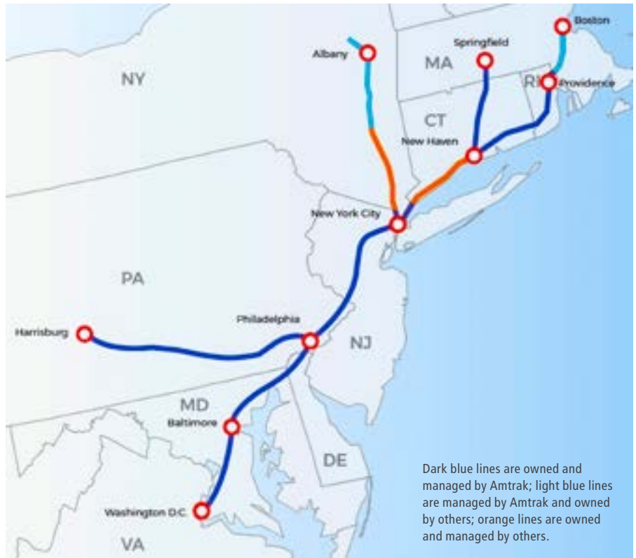
Figure 1: NEC Main Line and Branch Lines – Accountabilities
