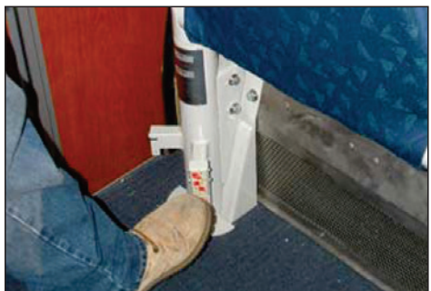
Figure 12-8 – Foot Operated Latch to Secure or Release the Bedroom Occasional Seat from Against the Wall
