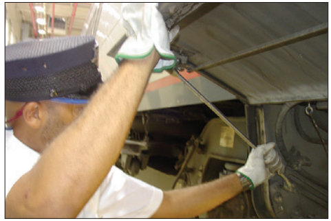
Figure 1-11 – Secure the door safety bar
