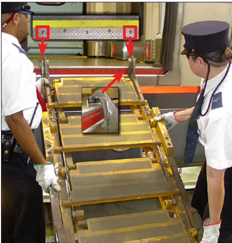
Figure 1-14 – Secure folding stairs to car body
