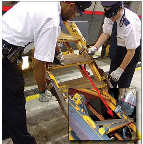
Figure 1-15 – Level stair steps
