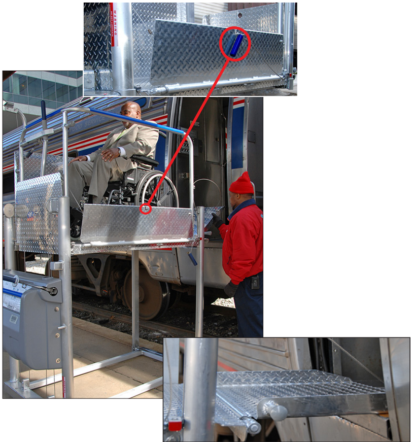
Figure 11-5 – Bridge Ramp Release Handle
