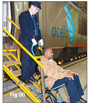
Fig (6) Roll chair onto folding stair. As chair starts to descend, slide hands to grip top of handle. Press down on handle for smoothest ride.
