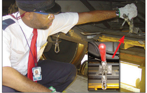
Figure 1-13 – Release folding stairs hold-down clamp
