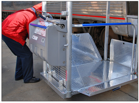
Figure 11-3 – Lowering Ground Ramp
