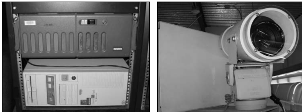
Figure 3. License plate reader (top on left) and LPR camera as installed in the Microscale Emissions Modeling System.
