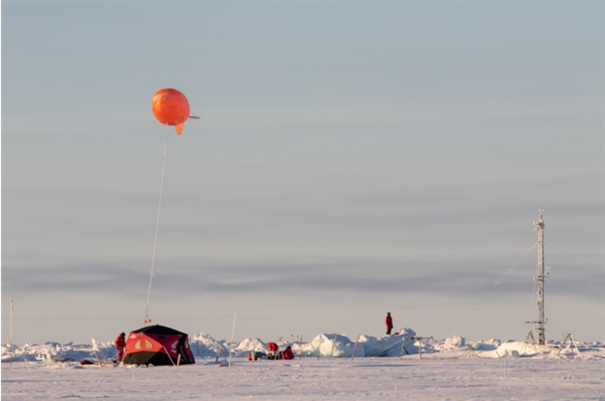
Fig. 4. Part of the MOSAiC ice camp in September 2020, with tethered balloon, meteorological tower, and other installations on the ice. (Photo: Marcel Nicolaus)
