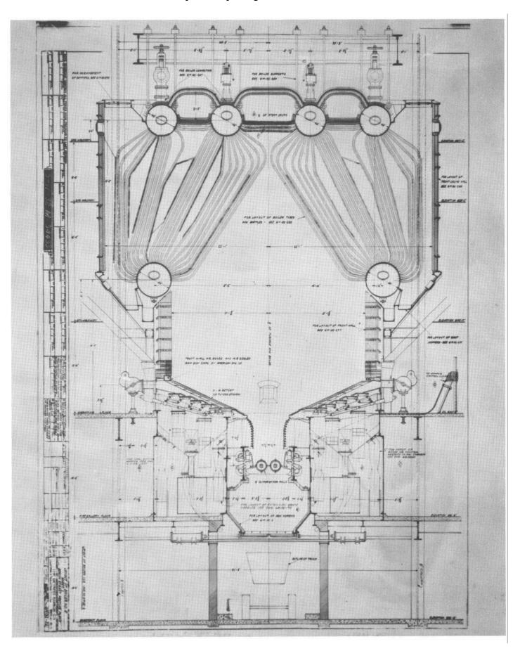
Layout of boiler No. 5 at the Beacon Street Plant. The boiler stands nearly 40 feet tall from the center of the boiler drums at the top to the operating floor below. approximately 240,000 gallons of water per hour are needed from the city water system for steam production.
