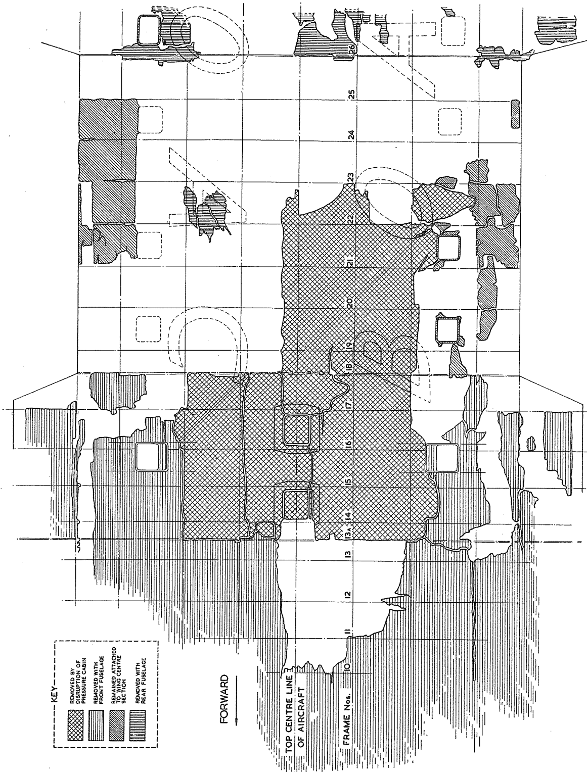
FIG. 18. DEVELOPMENT DRAWING OF WRECKAGE AROUND ADF AERIAL WINDOWS—G-ALYP.
