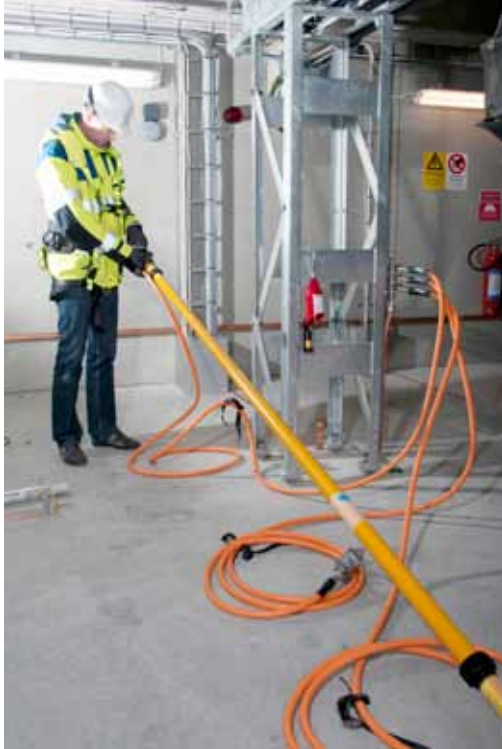
Three phase portable earthing device
