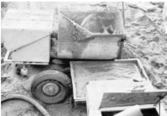
Figure 11. Step 1) Place water in mixer first. (66131)
