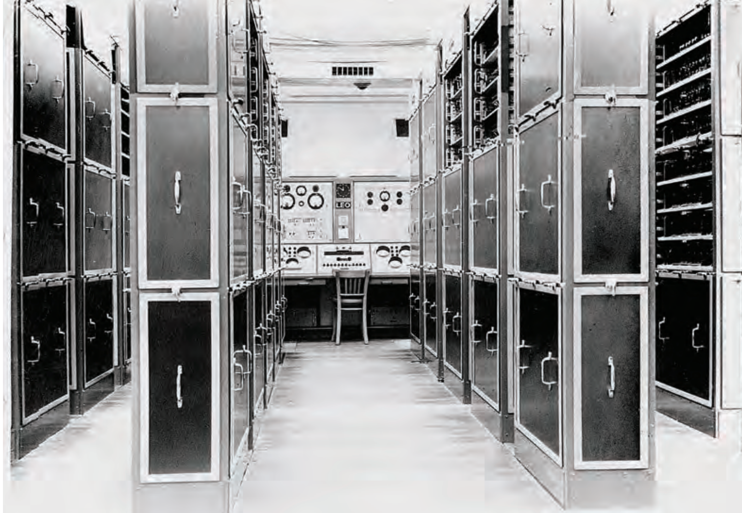
The operator's console of the LEO I electronic computer in the 1960s.
