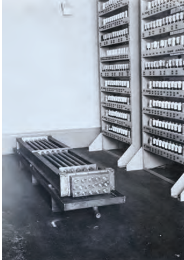
A complete memory battery, seen here in April 1948, consisted of 16 tubes (tanks) filled with mercury and sealed at each end with a metal plate into which quartz crystals (transducers) were embedded in intimate contact with the mercury.
