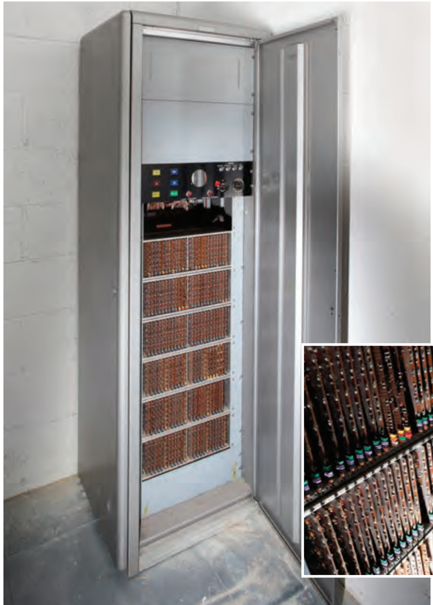
The Titan memory unit rack. The inset shows more detail.
