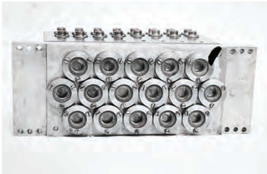
Below: End cap showing the 16 transducers embedded into the metal plate which was attached to the delay line tanks to make up a battery.
