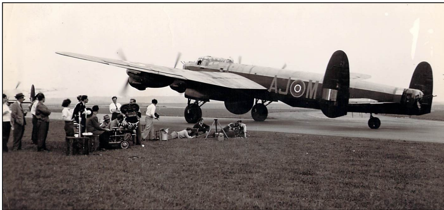
1954. Ground level filming of a Lancaster modified for the film, mid upper gun turret and bomb bay doors removed.
